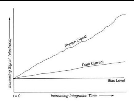
During an integration with a CCD, the bias remains constant, the dark current increases, and photoelectrons accumulate. At the end of the integration, you only know the total signal. To find the average photon flux, you must subtract both the bias level and the dark current from the total signal.
