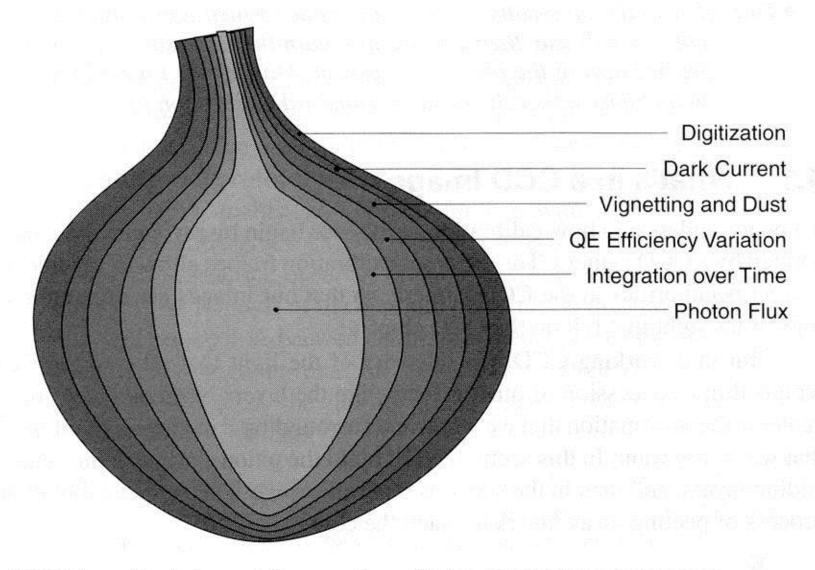
CCD information is layered like an onion, with the data that you really want—the flux of photons—hidden away in the innermost layer. To retrieve the photon flux, you must peel away unwanted signals and factors that influence the signal from the CCD. This process is called image calibration.
