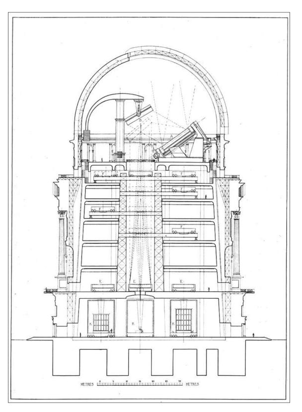
Figure 2- Ritchey's design for a 8 m fixed vertical Universal Telescope. Note the human figures that show the gigantic scale of this instrument. Adapted from Ritchey, G.W. (1929) *L'Évolution de l'Astrophotographie et les Grands Télescopes de L'Avenir*. Société astronomique de France.
