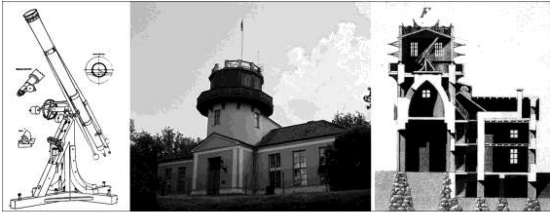
Figure 2- The great Dorpat refractor (left) was installed at Dorpat Observatory (center) under the rotatory cupola (right).
