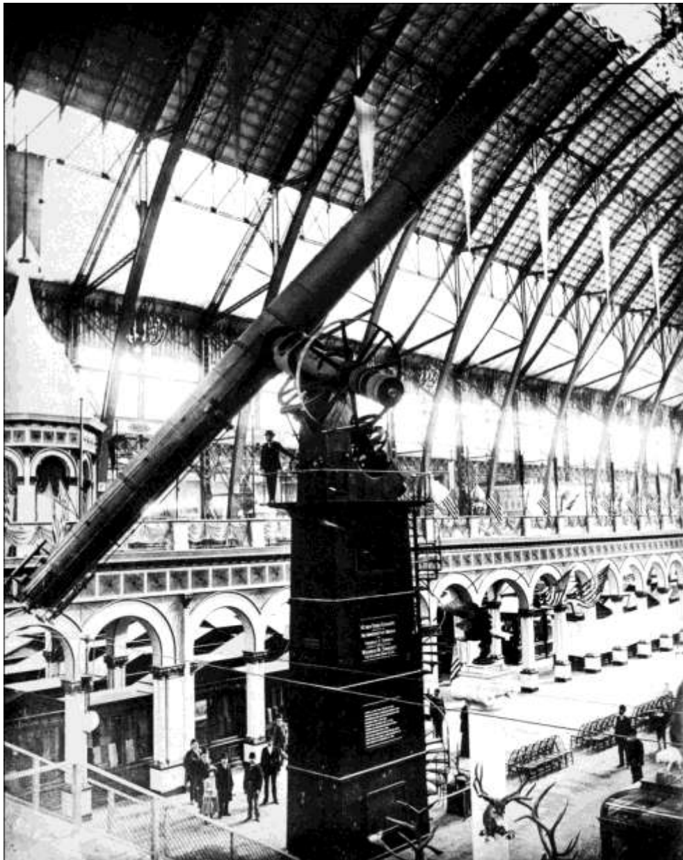
Figure 6- Mounting of the 40-inch Yerkes refractor on display at the Columbia Exposition in Chicago (1893).
