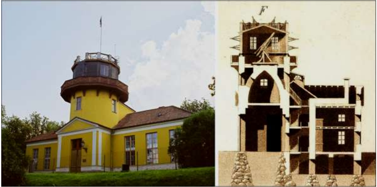
Figure 3- Dorpat Observatory main building (left) and cutaway drawing of the main tower with the great Dorpat refractor installed under the rotatory cupola (right).
