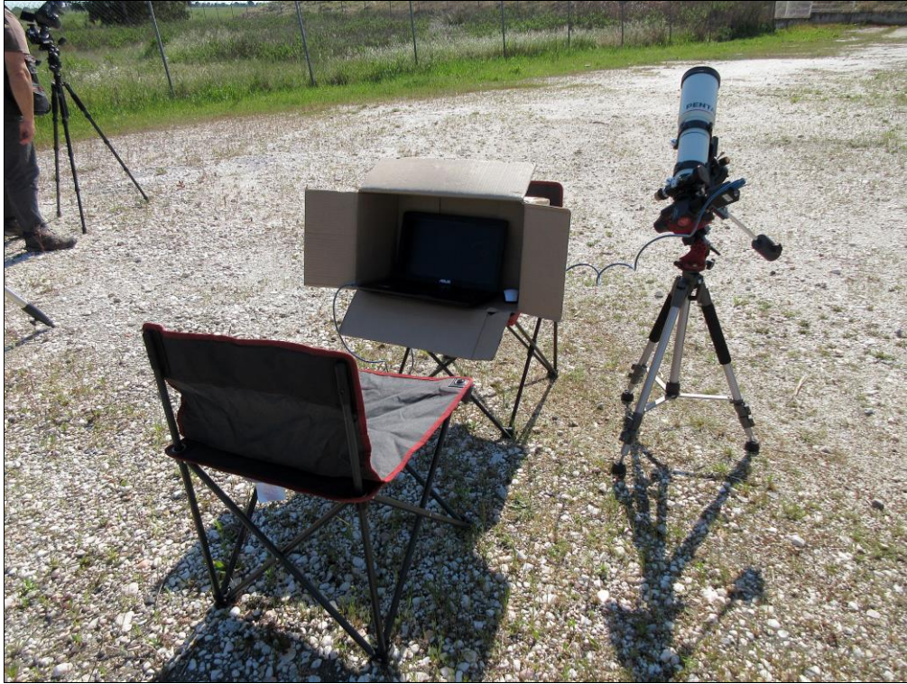
Figura 5- Pentax 75 SDHF F/6.7, Sky-Watcher Star Adventurer, GRASSHOPPER 3 2.8 MP MONO (GS3-U3-28S4M-C).
