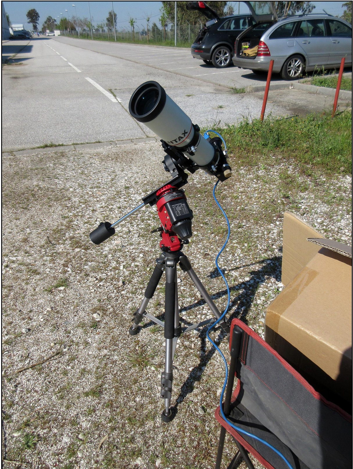
Figura 4- Pentax 75 SDHF F/6.7, Sky-Watcher Star Adventurer, GRASSHOPPER 3 2.8 MP MONO (GS3-U3-28S4M-C)
