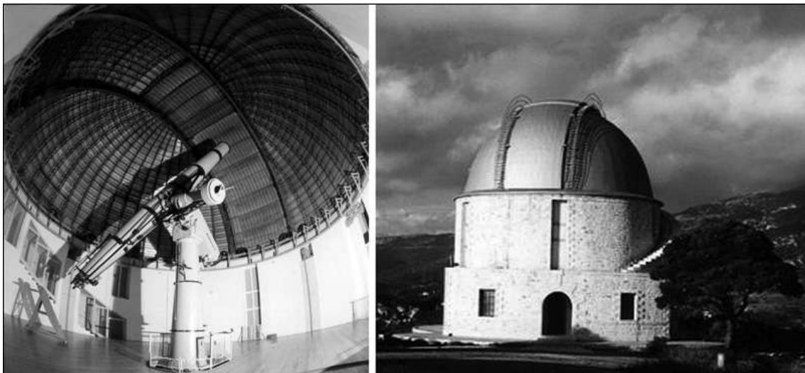
Figure 6- The Newall 25-inch refractor and new dome at the Penteli Astronomical Station (National Observatory of Athens - Greece).
