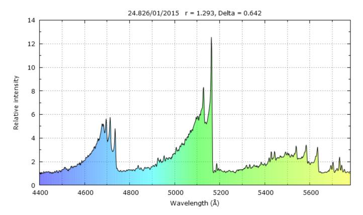
The first third of the most prominent Swan band with discerned fine structure (it need more resolution to resolve completely the rotational lines). High resolution spectrum by Christian Buil (eShel spectrograph, R ~11000). This is part of an excellent comet spectrum that span from 4280 to 7350A:
