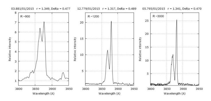
Basic structure of main C3 emission band. Since the difficulty of exciting C3 in the laboratory, identification of many lines is missing (lines attributable to this radical span from 3350 to 4700A). Spectrum by Christian Buil taken with a Lhires III spectrograph and 600 l/mm grating:
