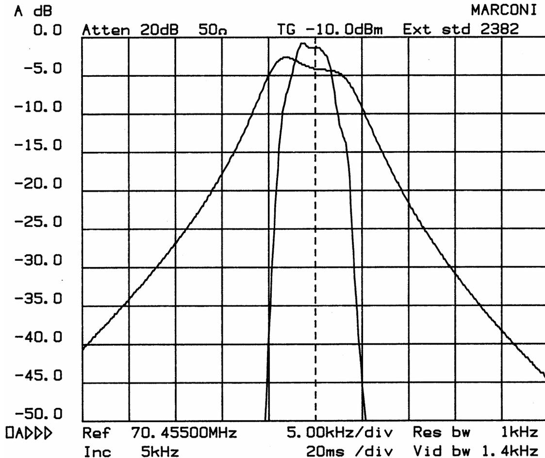
The wider trace is the unmodified RF board response and the narrow trace is after the Inrad mod is installed. There is a small increase in gain which has a slight effect on lowering the noise floor.
