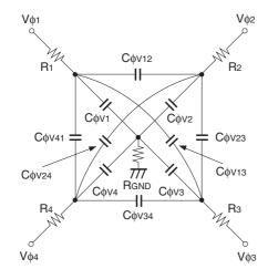
Vertical transfer clock equivalent circuit
