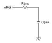
Reset gate clock equivalent circuit
