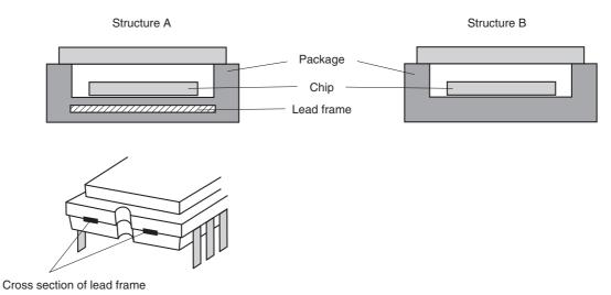
The cross section of lead frame can be seen on the side of the package for structure A.
