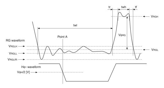
$\label{eq:VRGLH} \textit{VRGLH} is the maximum value and \textit{VRGLL} is the minimum value of the coupling waveform during the period from Point A in the above diagram until the rising edge of RG.$
