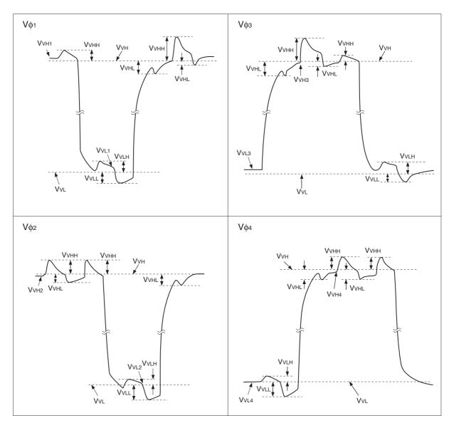
$V_{VH} = (V_{VH1} + V_{VH2})/2$
