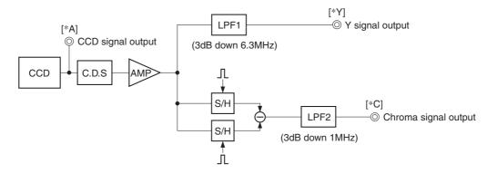
Note) Adjust the amplifier gain so that the gain between [\*A] and [\*Y], and between [\*A] and [\*C] equals 1.
