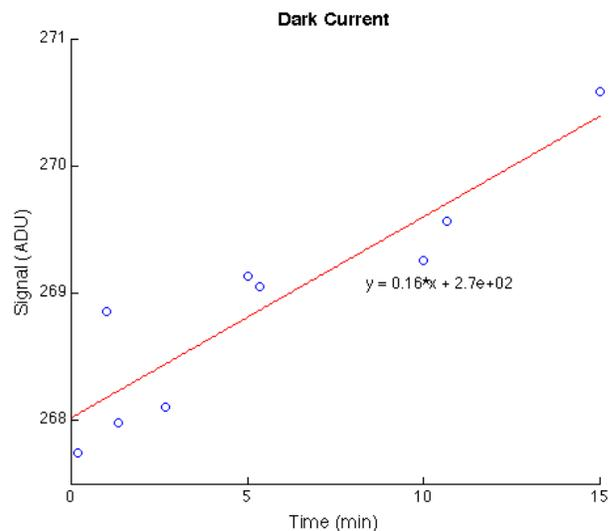
traction. A perfect dark frame will remove the constant current built up in the pixel, but the additional noise superimposed on this value (the random noise) cannot be pulled out. Thus, the less "bad" signal you have (dark current, light pollution, etc.) the cleaner your images will be.
