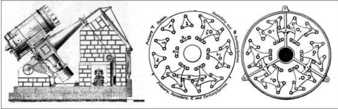
Figure 7- Equatorial Mount and mirror support of the Great Melbourne Telescope.
