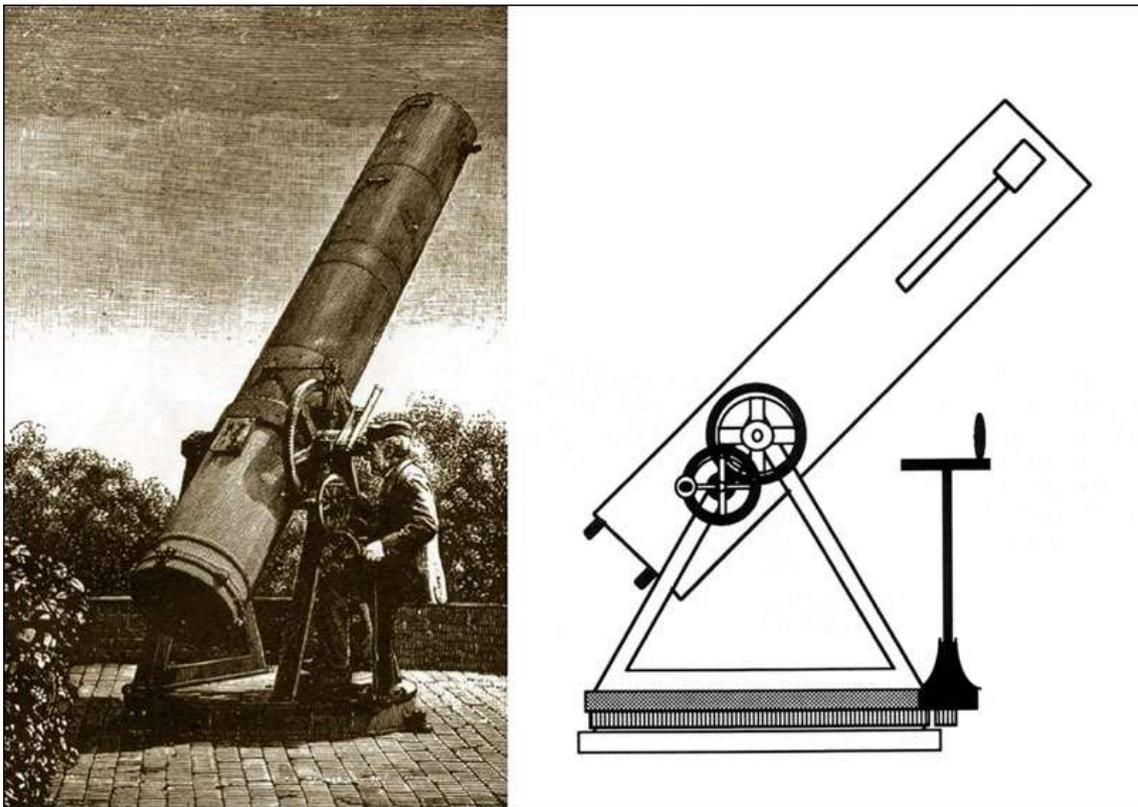
Figure 1- Nasmyth's 20-inch Cassegrain-Newton (around 1845) (left).
